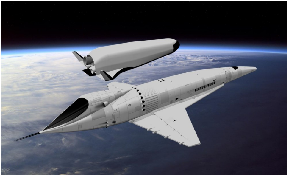
Figure 19: The 175-ft long fictional Orion III spaceliner and the 114-ft long conceptual Boeing TAV -112 orbiter are shown to the same scale. The TAV orbiter would have two versions: an unmanned cargo spacelifter and a passenger spaceliner. (Credit: J. M. Snead.)
