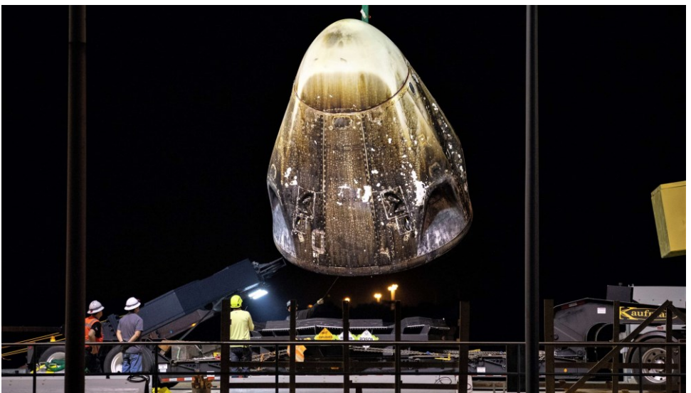
Figure 5: Return of the Crew Dragon Demo 1 capsule flown unmanned to the International Space Station. This was the capsule subsequently destroyed during a static ground abort system test firing. (Source: NASA)
