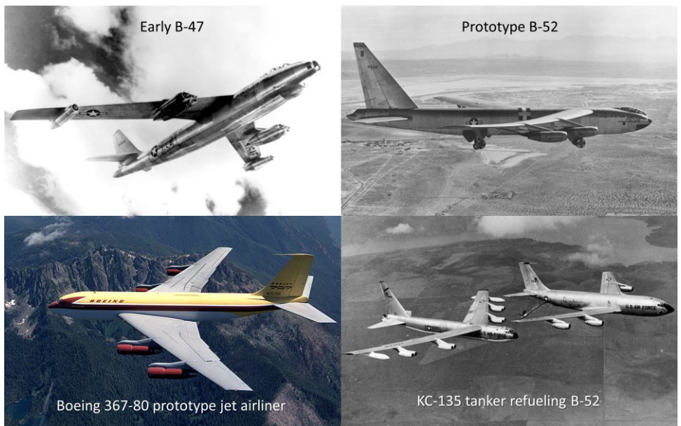
Figure 22: Development of the modern jet transport design. (Credit: J. M. Snead.)
