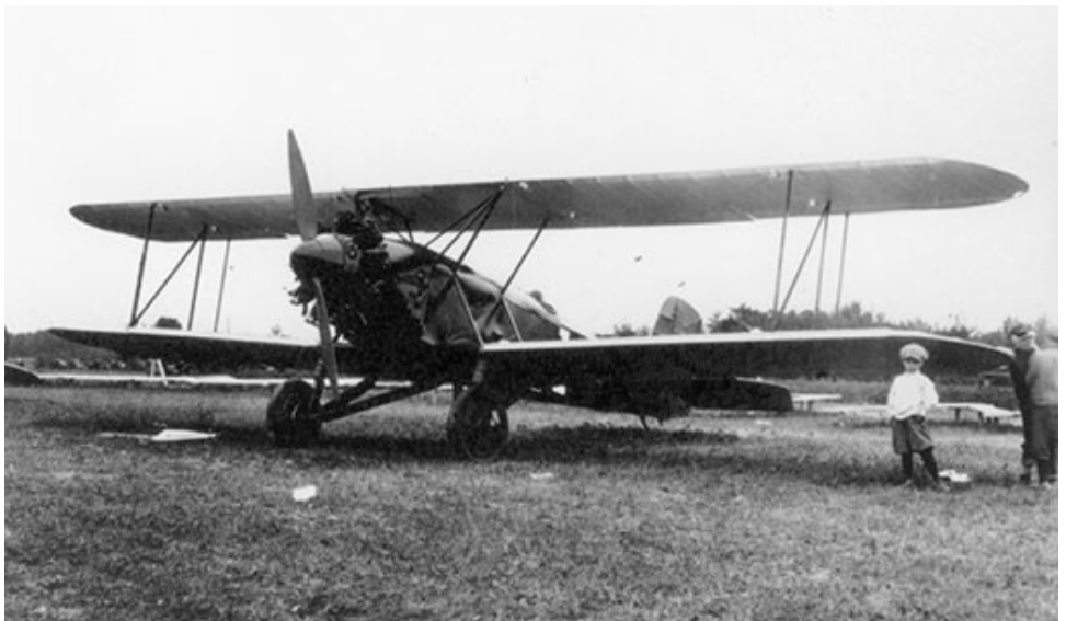
Figure 7: A Buhl Airster CA-3, a three-place open biplane was the first aircraft to receive an airworthiness certificate. (Source: NARA)
