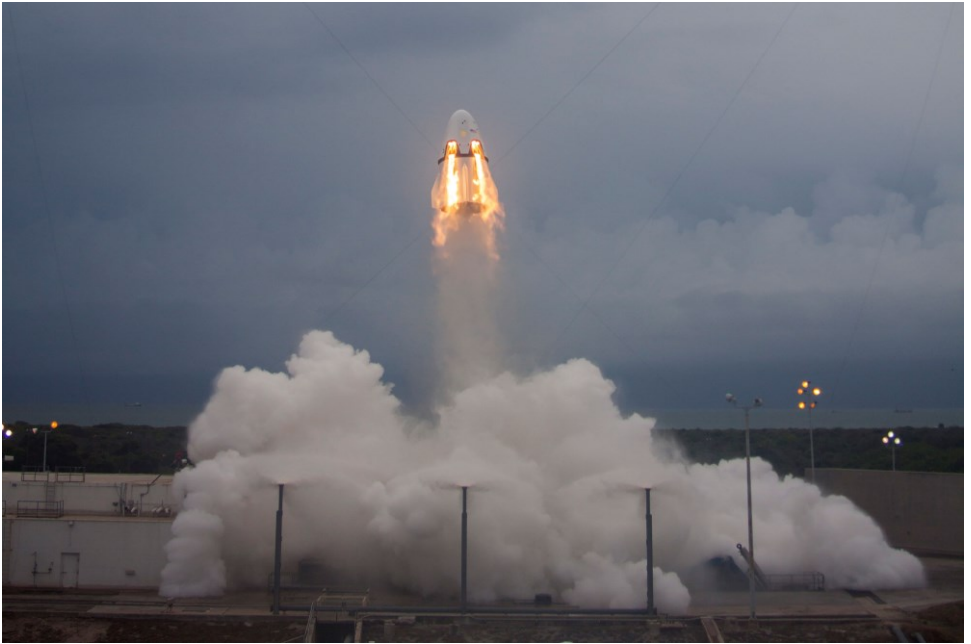
Figure 6: Earlier free flight test of the Dragon Crew abort system. This was a test capsule, not the flown capsule that failed. (Source: NASA.)
